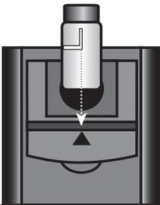
Insert the tube into the chamber, being sure to align the index line with the arrow on the meter. Close the lid. This tube is the sample
