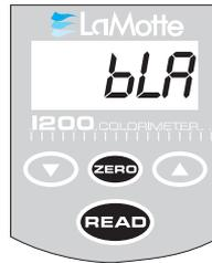
Push the **READ** button to turn the meter on. Press the **ZERO** button and hold it for 2 seconds until is displayed. Release the button to take a blank reading (0.0 ppm).
