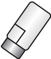
Cap and shake until powder dissolves. Wait 5 minutes for full color development. Solution will turn blue if phosphates are present. Wipe tube dry.
