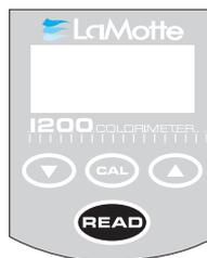
Align the index line with the arrow on the meter, insert tube into chamber. Close the lid. Push the **READ** button. Record results as ppm Orthophosphate.
