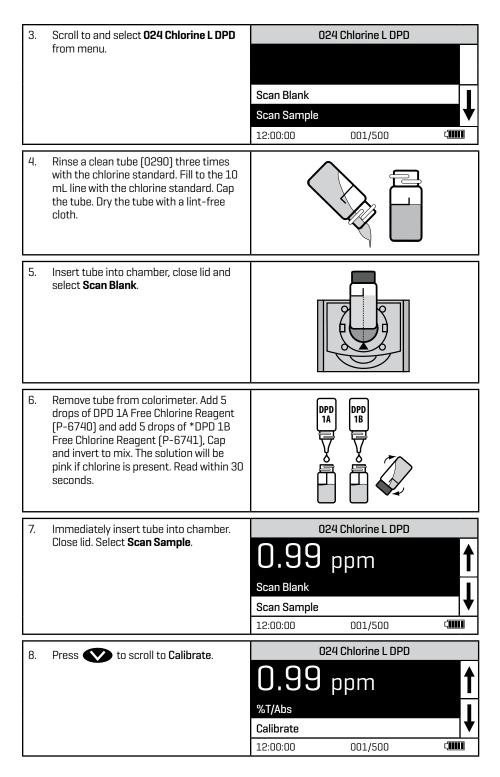
9. Press (NTE) to select **Calibrate**. A reverse font [light background with dark characters] will appear to indicate that the reading can be adjusted.
