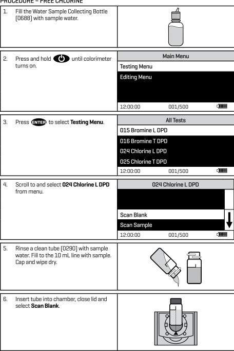
Remove tube from colorimeter. Add 5
