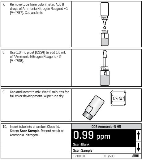
NOTE: The meter will remember the last scanned blank reading. It is not necessary to scan a blank each time the test is performed. To use the previous blank reading, instead of scanning a new one, scroll to Scan Sample and proceed. For the most accurate results, the meter should be blanked before each test and the same tube should be used for the blank and the reacted sample.
