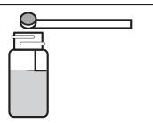
9. Cap and invert to mix until the powder dissolves. Solution will turn yellow if molybdenum is present.
