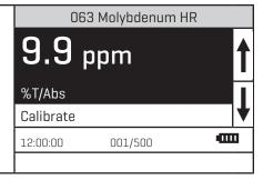
12. Press ENTER to select **Calibrate**. A reverse font (light background with dark characters) will appear to indicate that the reading can be adjusted.
