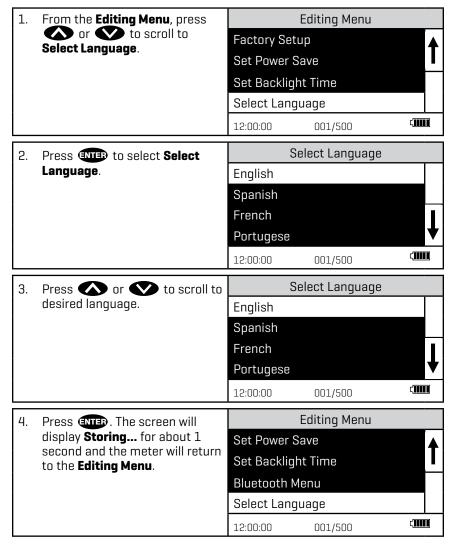
NOTE: If meter unintentionally switches to another language, use the procedure above to reset the meter to the desired language. For example, to reset the meter to English:
