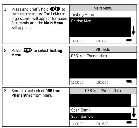
Rinse a clean tube (0290) three times with the iron standard. Fill to the 10 mL line with the iron standard. Cap the tube. Dry the tube with a lint-free cloth. 5. Insert tube into chamber, close lid and select Scan Blank. 6. Remove tube from colorimeter. Add 6 drops of \*Acid Phenanthroline Indicator [2776]. 7. Cap and invert 4 times to mix. Use the 0.1 g spoon (0699) 8. to add one measure of \*Iron Reducing Reagent (2777).
