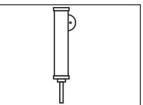
3. Use the 1.0 mL transfer pipet [2-2170] and pipette pump [30527] to add 1.0 mL of HR Reagent [3988] to each of 2 clean colorimeter tubes [0290].
