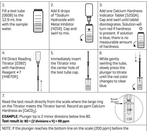
NOTE: If the plunger reaches the bottom line on the scale (200 ppm) before the endpoint color change occurs, refill the Titrator and continue the titration. When recording the test result, be sure to include the value of the original amount of reagent dispensed (200 ppm).
