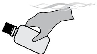
Tightly cap the bottle, and submerge it to the desired depth.
