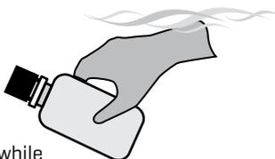
Replace the cap while the bottle is still submerged.
