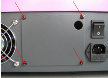
2. Loosen the 2 lamp-securing screws. Pull the bulb out and replace with a new lamp (12V 20W) of the same type. The filament type must be identical. Secure the new lamp with the locking screw. Tighten the screw firmly but do not over-tighten to avoid damaging or breaking the lamp.
