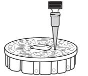
1. Fill any unused section of the disk using slow, even pressure. Add the sample water until the Blank Chamber is full and the Over Flow Chamber is partially filled.
