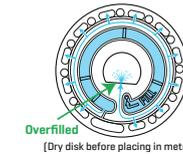
3. Do not under fill the disk. If the disk is under filled, the reagent chambers will not fill entirely and results will be inaccurate.
