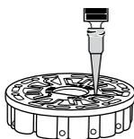
1. Fill any unused section of the disk using slow, even pressure. Add the sample water until the Blank Chamber is full and the Over Flow Chamber is partially filled.
