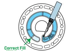
2. Do not overfill the disk. If the disk is overfilled, sample water will flow out of the overflow hole in the center of the disk. The disk is not leaking. Dry the disk and run the test.
