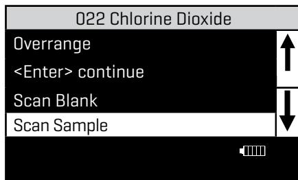
**CALIBRATION** As with all pre-calibrated meters, it is highly recommended, even if not required by regulations, that the user periodically verify the performance of the meter by running standards with a predetermined concentration. Results outside of specification are an indication that the meter needs to be adjusted. This can be done following the calibration procedure.
