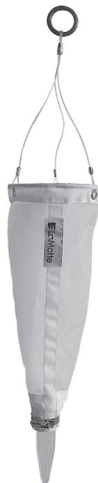
collect the plankton. In most cases the pore size of the net is small enough to retain the plankton and concentrate them into the conical collecting tube at the end of the net while the water is filtered through the net.
