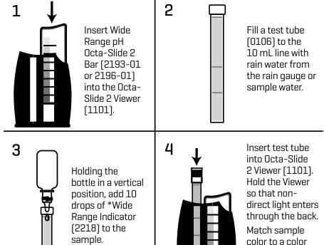
NOTE: If the color observed in your sample is between two colors on the comparator, the value may be reported to the nearest 0.25 pH unit. If the color produced by your sample is not in the range of the color standards in the comparator, use the following chart to estimate the pH of the sample:
