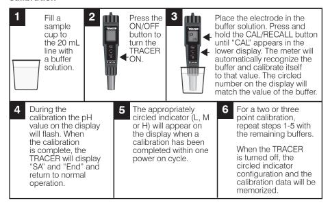
NOTE: If the buffer solution is more than 1 pH unit off from 4, 7, or 10, or the electrode slope is low, the meter will assume that there is an error and the calibration will be terminated. END will be displayed.
