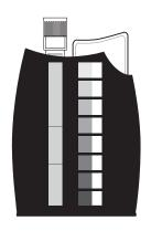
The Octa-Slide 2 Viewer should be held so non-direct light enters through the back of the Viewer. Insert the reacted sample into the top of the Viewer. Slide the Octa-Slide 2 Bar into the Viewer and match the color of the reaction to the color standards.
